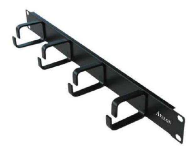
**Avalon** Horizontal Cable Managers with rings are capable of managing cables on the front and rear of any standard EIA 19" rack or cabinet. These Panels are constructed of a steel panel with plastic D-rings attached. Horizontal D-rings shall snap into panels and vertical D-rings shall be screw mounted to rack. Horizontal panels shall have pass-through holes and shall be available in both front and rear versions and front only versions.
