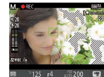
To ensure the best results in movie shooting, the D7200 has a handy feature that uses "zebra" patterns to indicate areas at risk of blown-out highlights. This can be quickly accessed via the "Z" button, and can be set to not record the "zebra" patterns when outputting to an external HDMI recorder.
