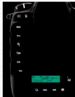
When shooting where light is scarce, the D5's button illumination provides enhanced visibility of the camera controls. The release mode dial and major button icons on the rear and upper-left sides of the camera can be lit with LED transparent illumination, as well as the top and rear control panels. The playback and delete buttons can now also be illuminated.
