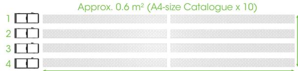
The Quad Filter System Plus consists of four very large, thick accordion filters. It provides exceptional protection from dust and dirt, and is a simple system that is easily maintained for the life of the projector.
