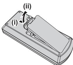
2. Remove the batteries.
