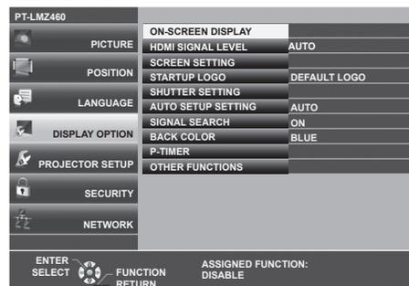
4) Press ▲▼ to select the desired sub-menu item, press ◀▶ or the <ENTER> button to switch or adjust settings.
