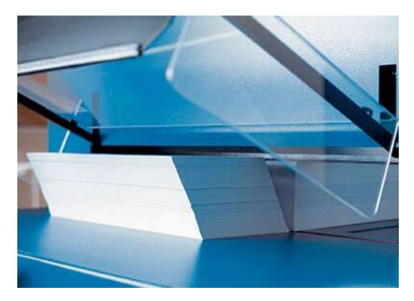
Model 842 offers an adjustable paper guide and models 846 and 848 feature a spindle driven, self-locking backstop for extreme accuracy and convenience during repetitive cuts. These cutters can be mounted on any secure table surface although the optional floor stands are recommended for proper cutting height and leverage. Dahle Stack Cutters are manufactured in Germany and can be found in art departments, custom frame shops, and print & copy centers throughout the world.
