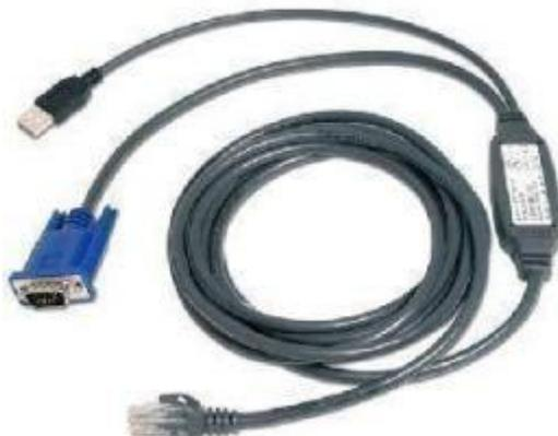
The USBIAC2-10 supports USB 2 peripheral devices (Virtual media & Smart card/CAC) on Avocent Mergepoint KVM switches.
