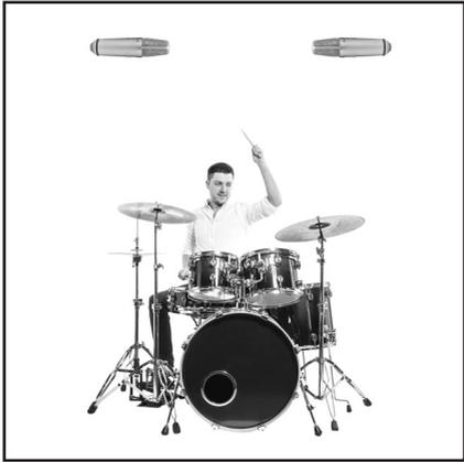
In this diagram, two WA-87 R2's are used in a spaced pair configuration to record stereo drum overheads, maintaining equal distance from the snare drum for proper phase.
