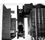
Tool-free, snap-on fan cover helps installing fan simple, easy and quick.
