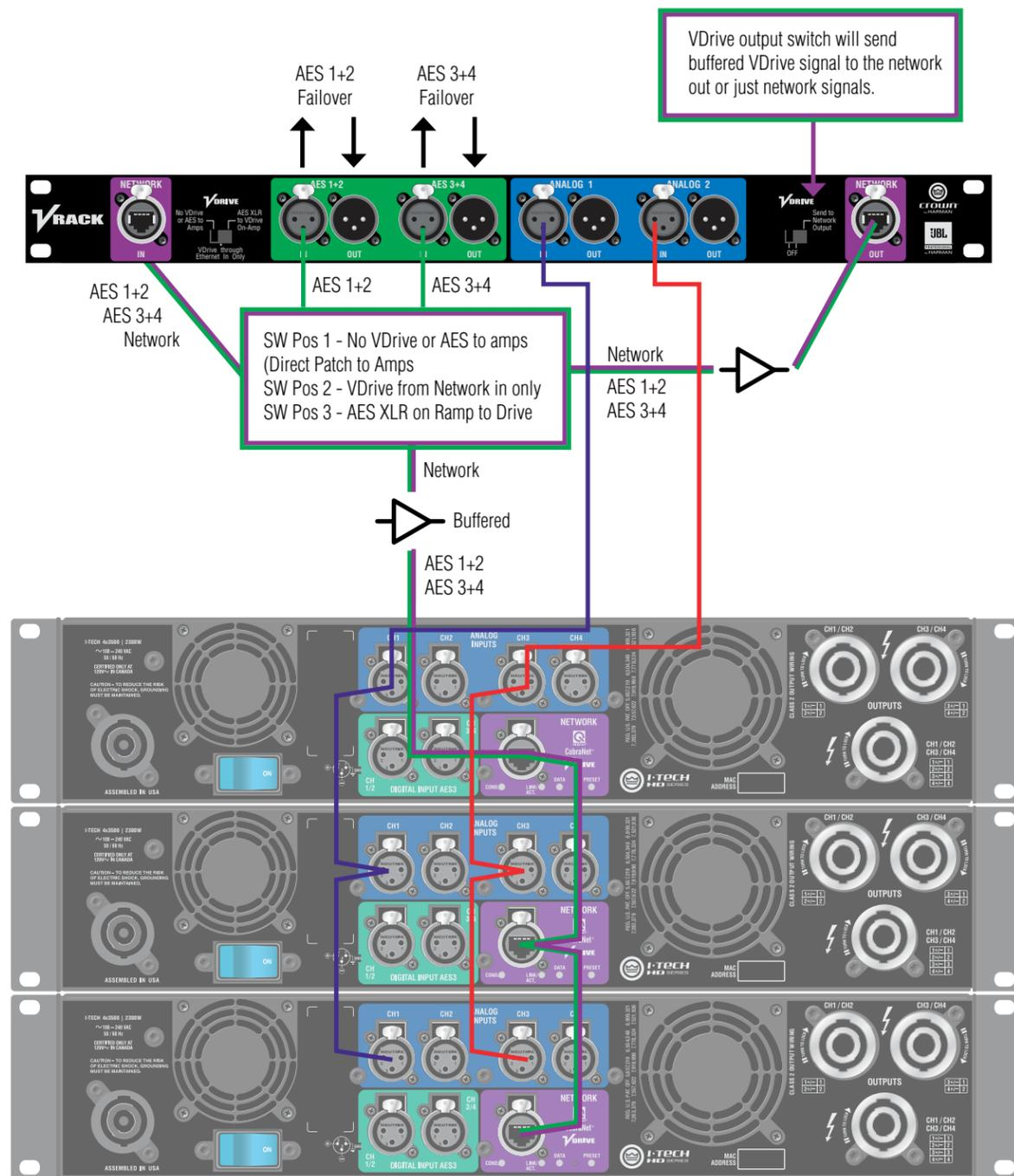
\*\*\*Please note, the AES3 signal is distributed via VDrive from the input panel to the amplifiers. Therefore, any time AES3 is patched directly to the input panel, VDrive must be enabled via the software or front panel display of the amplifier for the AES3 signal to be seen by the amplifier. (see page 21 for more details)
