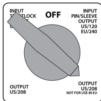
Switch Position "Input Pin/Sleeve, Output US/208" provides 208VAC Operation from the Cee-Form pin and sleeve connector. From an external power distribution system, send 3 phase 120VAC power to the X, Y, and Z pin of the Cee-Form connector and the VRack will operate in 208VAC operation mode. Each I-Tech HD amplifier will see a dedicated line-to-line connection as well as ground. In "Input Pin/Sleeve, Output US/208" mode, the end user is able to link 2 VRacks together. Amp 1 = X, Y, and GND
