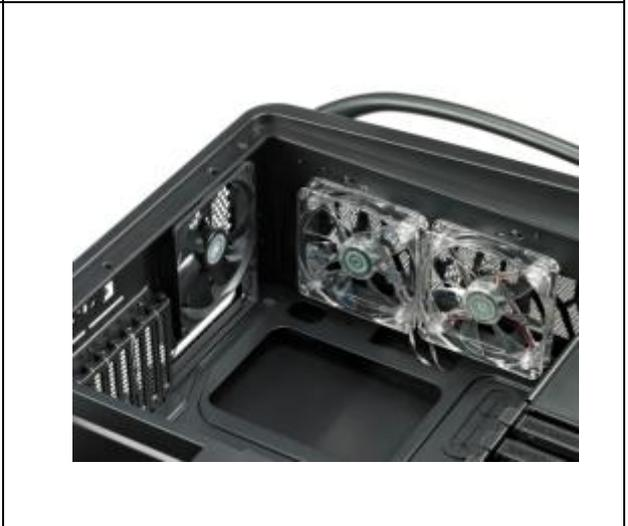
Can install 140mm fan x 2 at top
